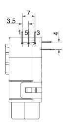
Remark:(1)In case of no tolerance shown in outline dimension:outline dimension≤1mm,tolerance should be±0.2mm;outline dimension>1mm and <5mm,tolerance should be ±0.3mm;outline dimension≥5mm,tolerance should be ±0.5mm.
